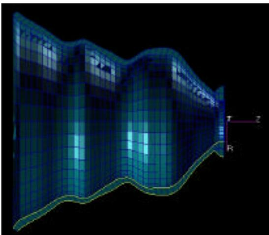
Hourbell6 – full bell again but ignoring the results for the small bell in the optimisation. The large bell is then rescaled to replace mistuned small bell. The results of this design iteration are shown in the table below.
