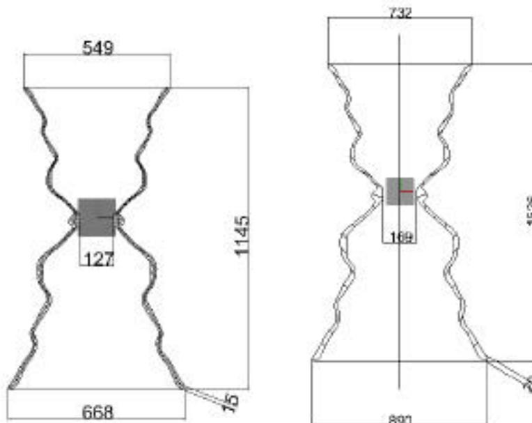
Final profile at original scale and scaled up (left) to produce the pitches E3, G#3, D4
